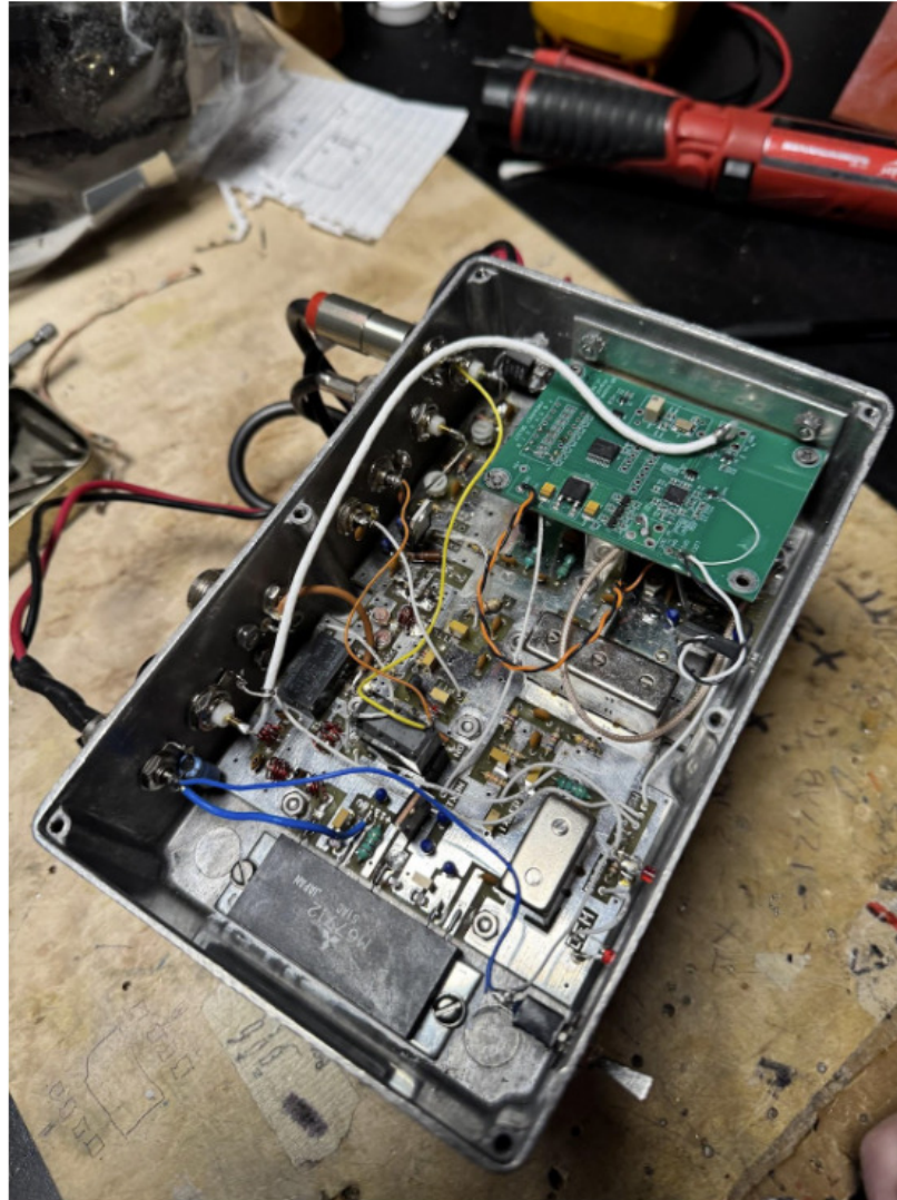
DigiLO Board installed in the 222 Mhz Demi Transverter Thanks to Ray N3RG
